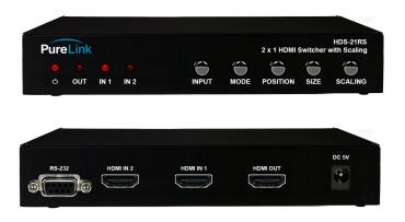
The HDTools HDS-21RS is a 2-HDMI input to 1-HDMI output switcher and scaler providing easy switching between two HDMI source signals to a single high definition display. The HDS-21RS features auto-scaling of any video signal up to 1080p, as well as PIP (picture-in-picture) technology offering built-in multi-view functionality.
